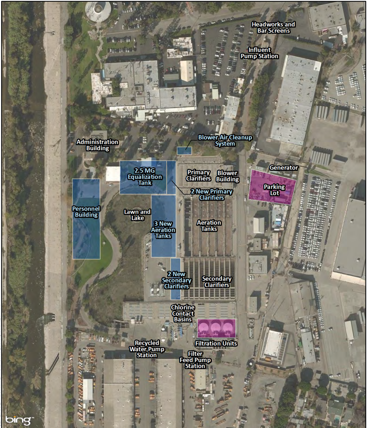
Figure 7.22 - Potential Process Location for Concept Option #17 (LAGWRP to Headworks Reservoir) One Water LA 2040 Plan Summary Report
